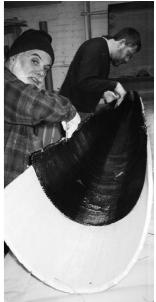
Ted Warren (front) and Ted Grossbart (rear) laying up the inner carbon skin of the new bow section prior to vacuum bagging.
