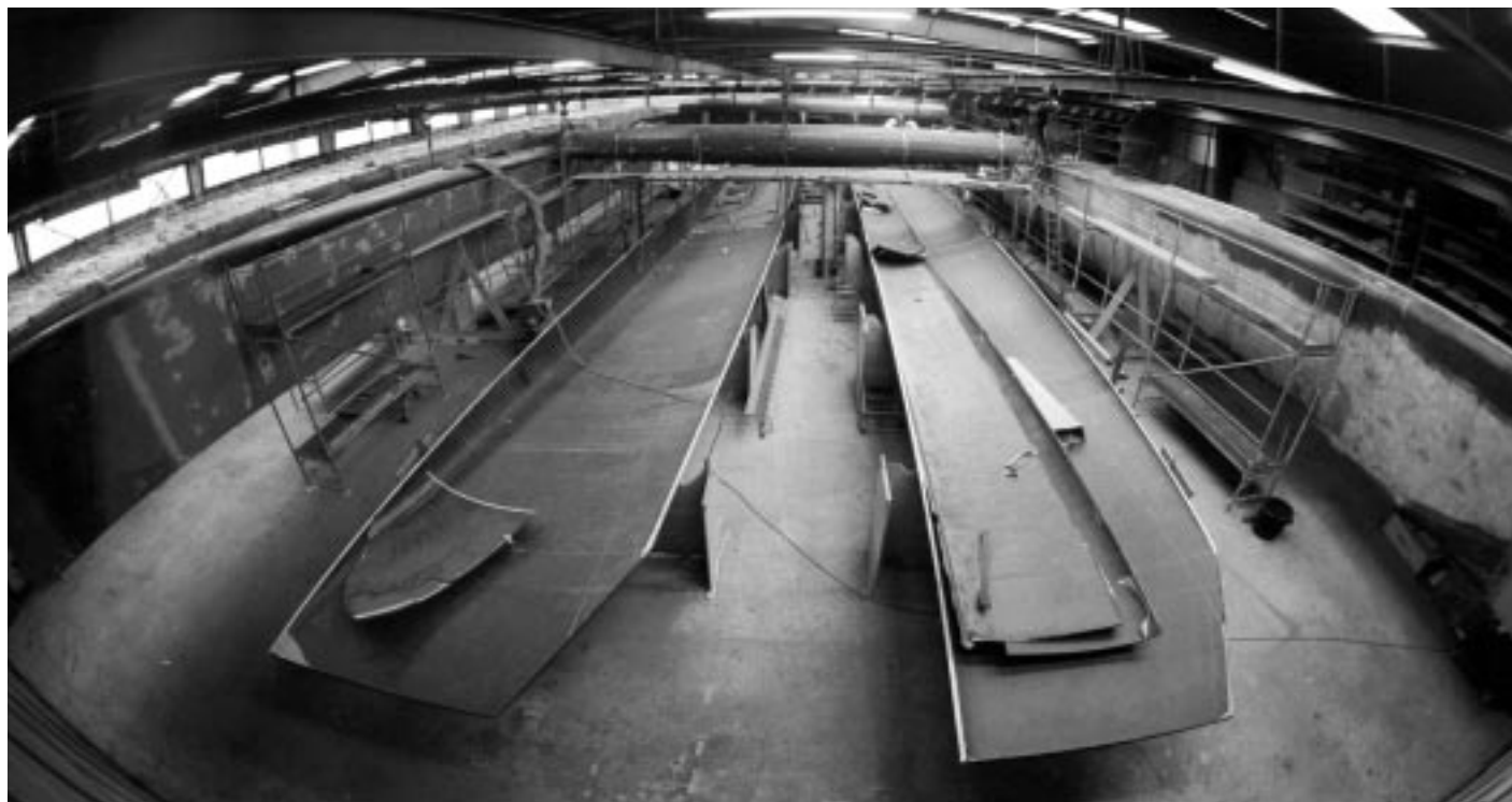
Two sections of a hull for a 100'+ multihull recede into the distance at the Multiplast workshop.
