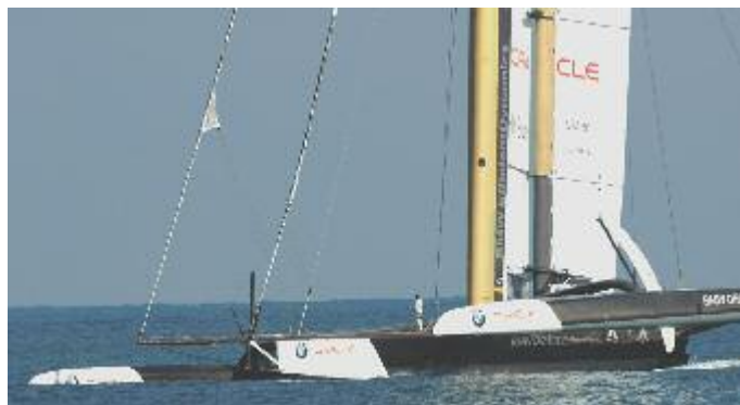
BMW Oracle foredeck and wing mast. Note the pressure sensor port, gearing for the wing mast and longer amas than center hull.
