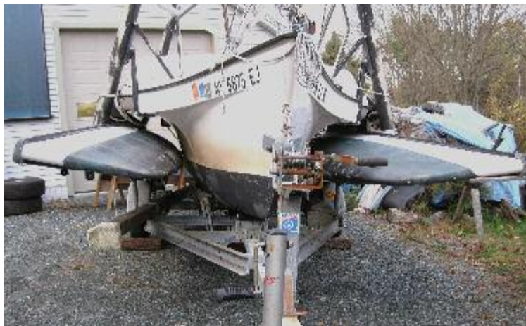
Tramp parked in its new home in West Hartford, VT, showing a view of the Farrier folding system which, though improved over the years, still retains the basic principles used on the Tramp.
